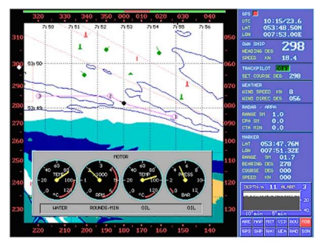
If the motor fails in pressure, temp. etc (too high or too low values) the motor instrumentation will be shown automatically. If you want to control the motor anyhow, you press button 3.
